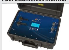
FILTERTECHNIK says its Particle Pal is a self-contained portable measuring system that gives ISO, NAS and SAE Cleanliness readings and the option of water content analysis for oils and/or diesel fuels, complete with a re-chargeable battery, high pressure internal gear pump and controlled flow rate. Whether on-site or in the laboratory, the Particle Pal can provide cleanliness readings in real time to allow an Engineer to fully understand the condition of their oils or fuels
